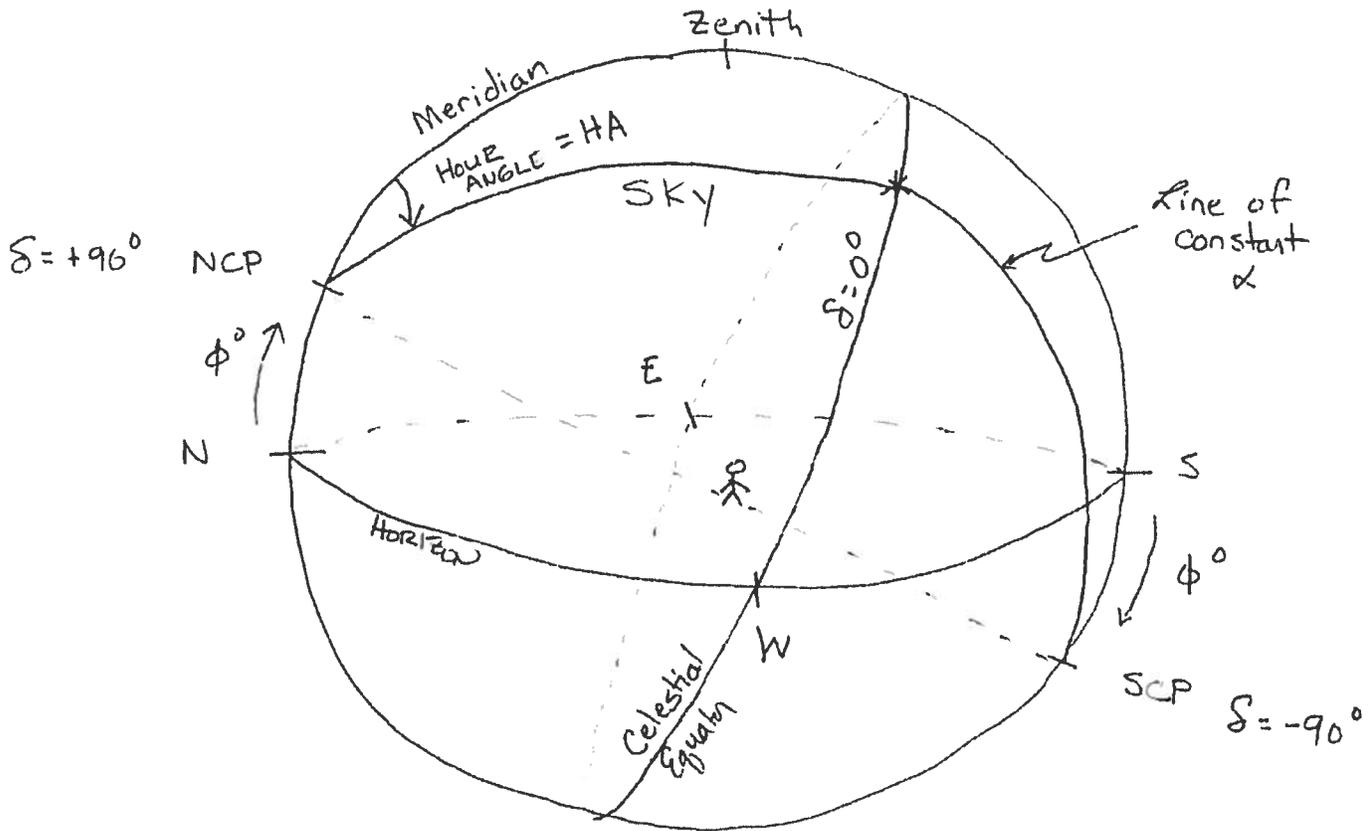
Hour Angle  $\equiv$  HA  $\equiv$  the angle between the meridian and the line of constant  $\alpha$  going through a source.
